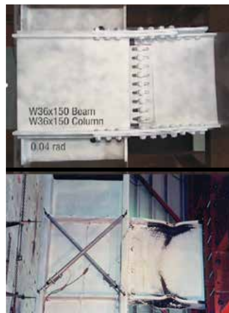
Figure 1: Experimentally-tested DuraFuse Frame (top) and Reduced Beam (bottom) moment connections.
