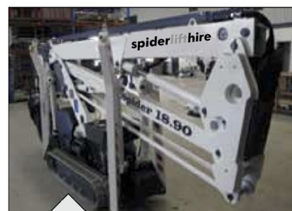
With the tracks retracted, the 18.90 has an incredible stowed dimension of only 792 x 1951 mm which allows it to drive through a domestic doorway!
