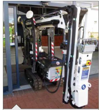
The light-weight basket is simple to remove in less than one minute, allowing very narrow access and a stowed length of only 3.69m
