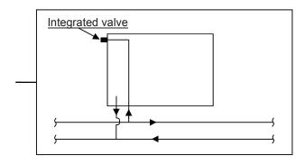
Note: Air bleeds **MUST** be in one of the top connections of the radiator. Radiators **MUST** be installed level and vertical.
