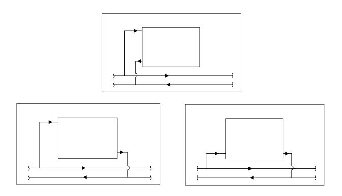
Typical Method of Plumbing a Compact Valve 6 Port Radiator
