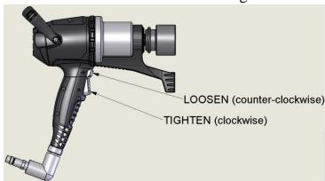
4. The final air pressure must be set after the tool has stalled on the first bolt with the trigger depressed. The stall point is reached when there is no longer any movement of the nut and there is a constant flow of air through the motor. After setting the final air pressure, the regulator can be locked by depressing the knob until it clicks, this will ensure the pressure remains at the set point for the required torque value.
