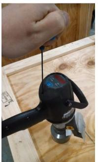
Use T-handle to remove the (3) screws that hold the rear cover on the tool.
