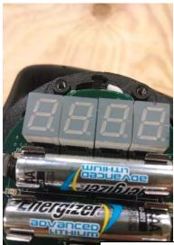
Carefully remove batteries with your fingers. (Do not use any conductive items to pry the
