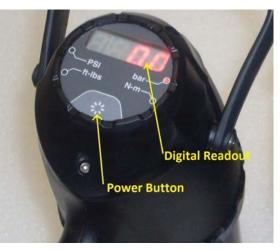
To activate the digital readout, push the power button once. The display should turn on. At this point you will get to choose whether you want to see (PSI/ft-lbs) or (bar/N-m). To switch between the two, the button must be pushed and held for two seconds. The light will switch to the other side. To switch between PSI and ft-lbs, or bar and N-m, push the button once while the display is on.
