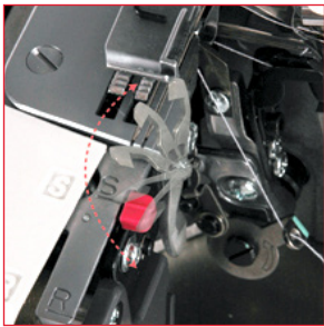
Easily Retractable Upper Knife
