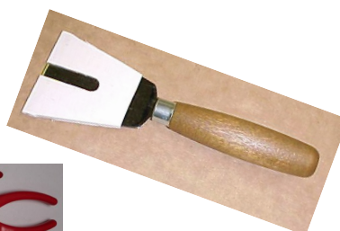
WDD 630 Trim Plate Knife (First CUT of the Weld Rod)
