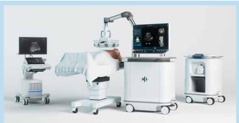
The Edison Histotripsy System, developed by Histosonics, is displayed in the photo above. The screen on the left shows real time imaging of the tumors as they are being dissolved. The arm on the device to the right is positioned over the patient to direct the ultrasound.
