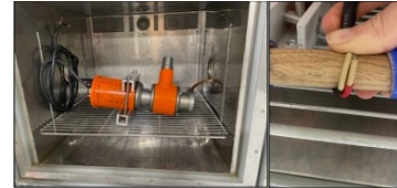
Pump Installed in Cold Chamber and Wire Testing
