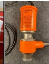
Pump Before and After Salt Fog Testing
