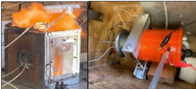
Pump During Ignition Protection Testing and Explosive Mixture Verification
