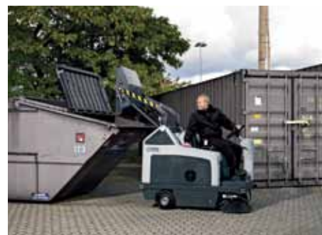
The high capacity hopper holds up to 130 litres of dirt, and is able to dump it to a height of 1.37 m
