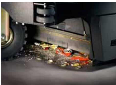
Collection of large debris without the operator having to stop the machine and pick it up manually
