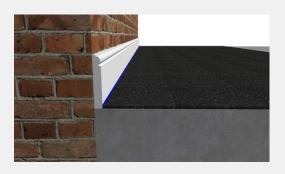
**4.** Lay the ImpactoMat up to the Perimeter Flanking Strip and into the adhesive, pressing from the centre outwards to exclude air and ensure overall contact with the adhesive.
