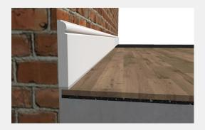
**6.** Install your final floor finish as per the manufacturers instructions installing perpendicular to the ImpactoMat joins. Once this is fitted trim off excess perimeter strip or fold over floor layers to place skirting board on top and trim off excess. Seal perimeters with an acoustic sealant.
