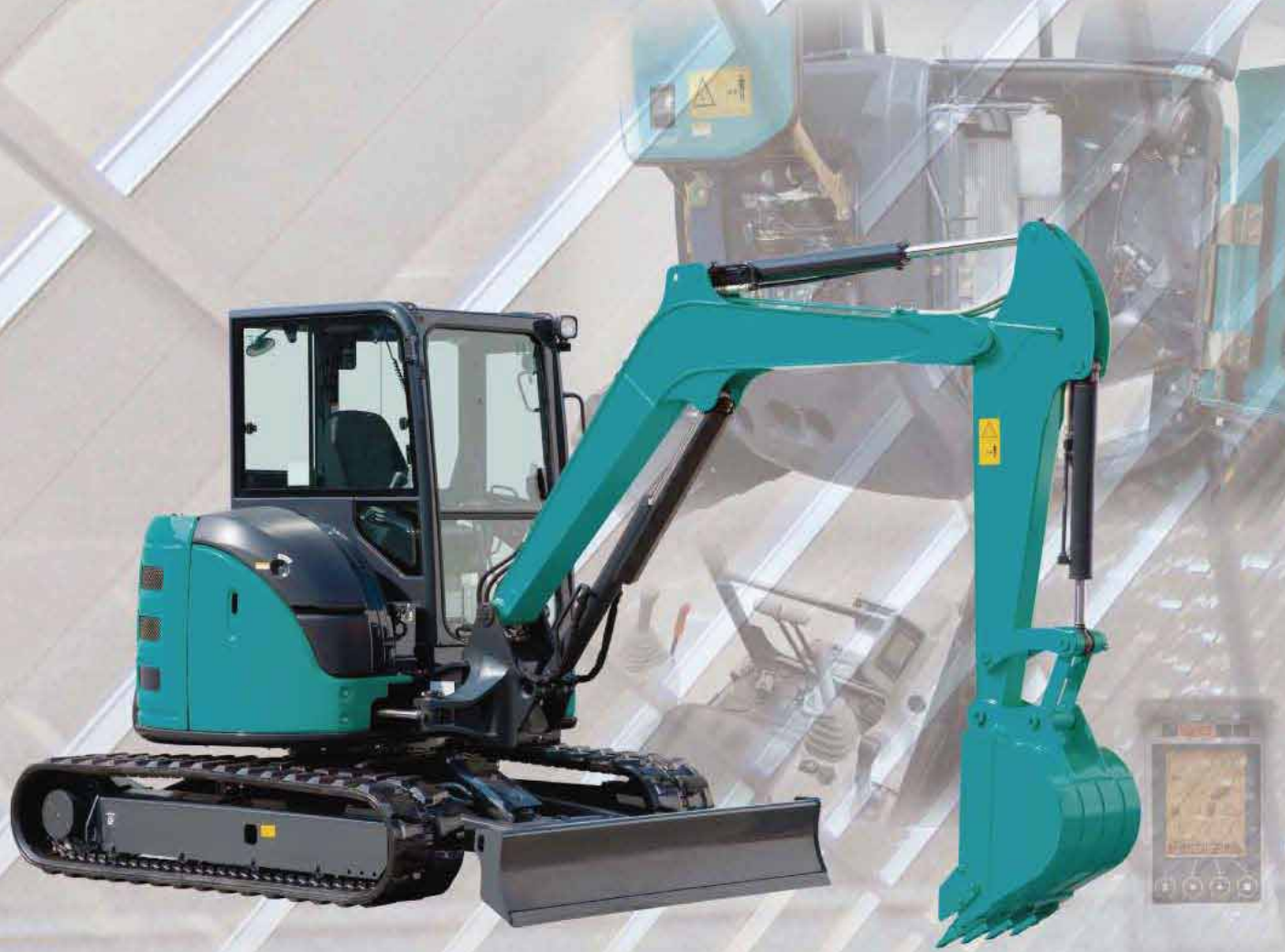
AX33U-6A Operating weight 3,130kg Capacity 0.09m 3 Rubber shoes, 4-pole canopy
