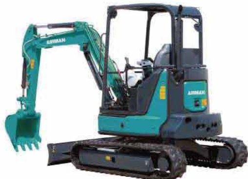
AX33U-6A Operating weight 3,130kg Capacity 0.09m 3 Rubber shoes, 4-pole canopy
