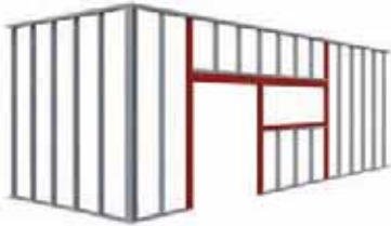
Openings in external walls
