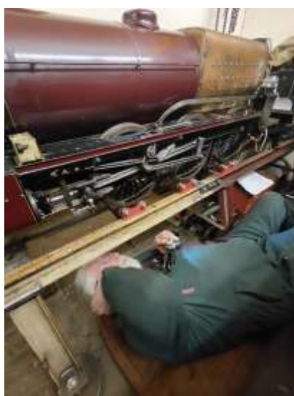
The Royal Scot has been having work done to update parts, 2 new lubricators have been fitted along with new pipework and superheaters in the smokebox.
