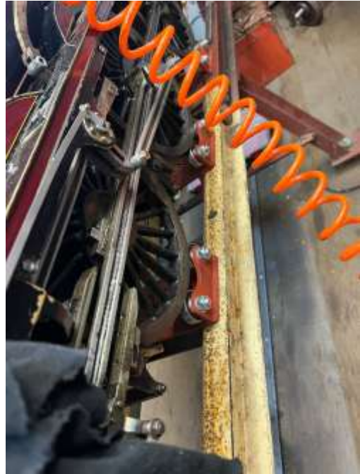
The Royal Scot on a rolling road. Fitted with an air compressor to check valve timing is in the right place, amongst other things.
