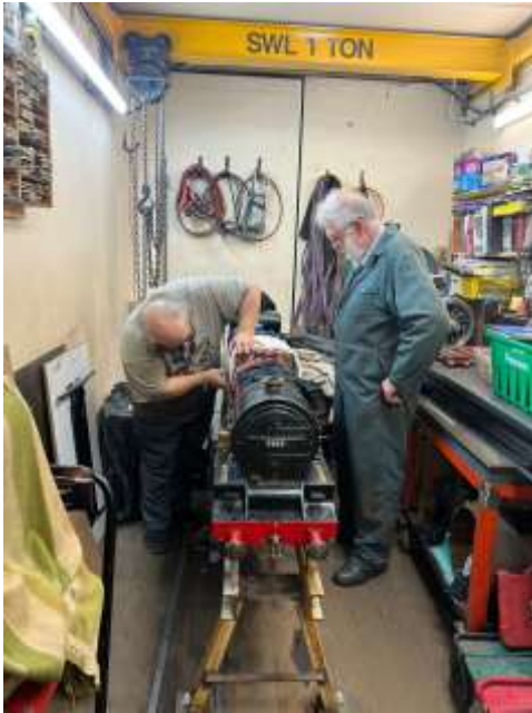
John and John working on the boiler lagging to the Royal Scot
