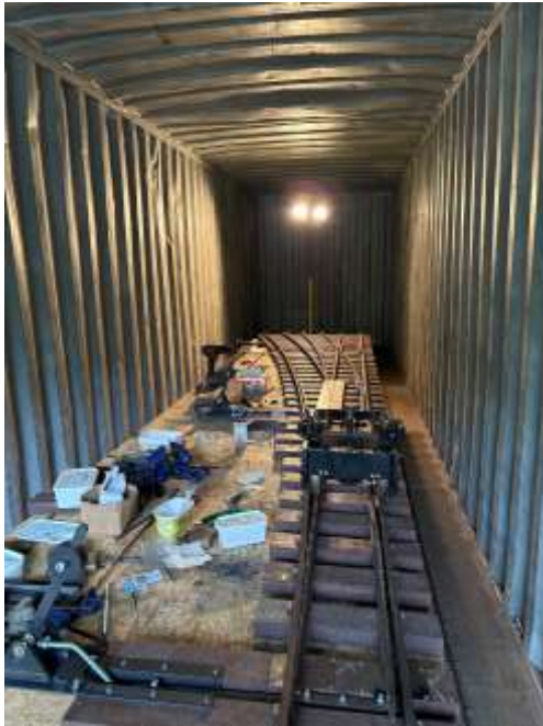
Point completed and tested with the spare '300' Bogie
