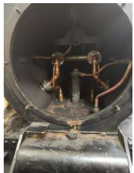
The Royal Scot has been having work done to update parts, 2 new lubricators have been fitted along with new pipework and superheaters in the smokebox.
