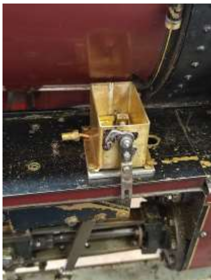
The Royal Scot has been having work done to update parts, 2 new lubricators have been fitted along with new pipework and superheaters in the smokebox.
