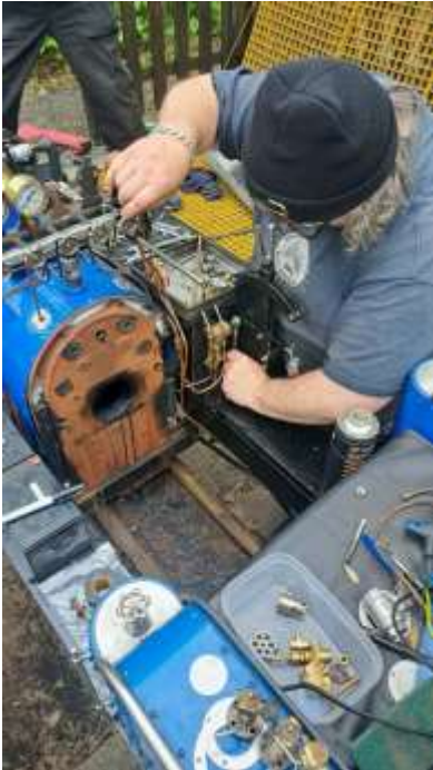
The pipework being reconnected on the Shay
