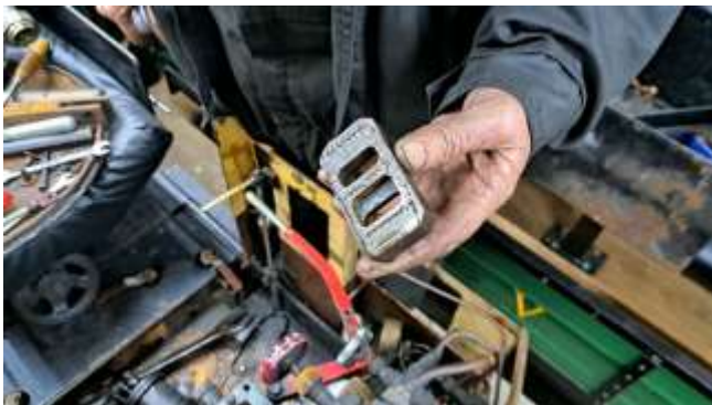
Phil has been lapping in the regulator valve on the Garratt, both pilot and main valves had been weeping steam through when the regulator was closed, so this work should make a noticeable improvement.
