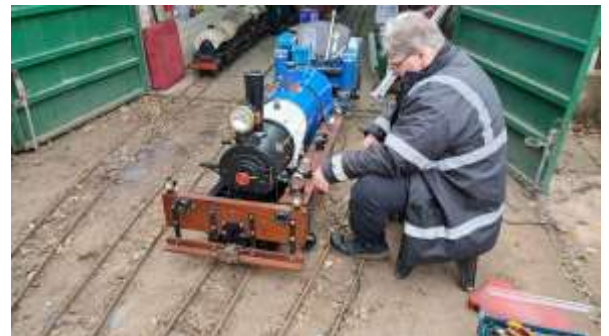
Reassembly of the freshly repainted boiler tins continues now that the engine has been refitted, and Jason has been looking at what's required for rewiring.
