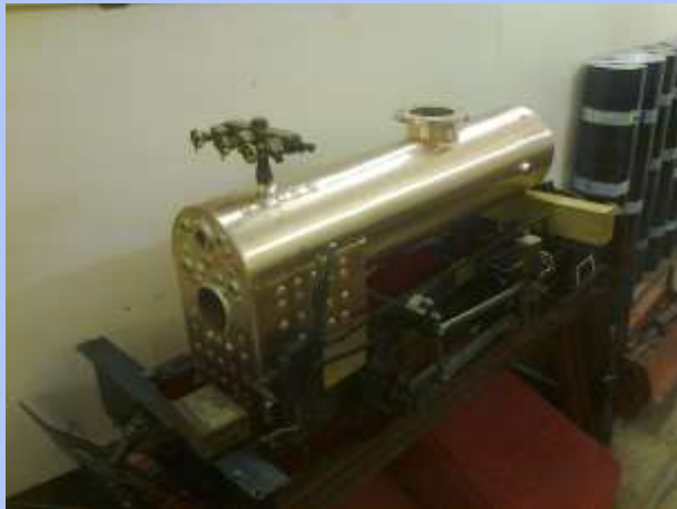
Dr John's new boiler arrives and is trial fitted into the chassis.
