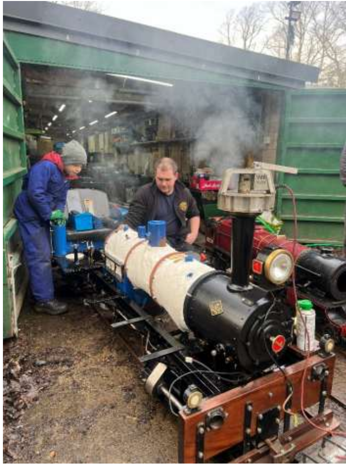
Conor lighting a fire to assist the descaling of the boiler
