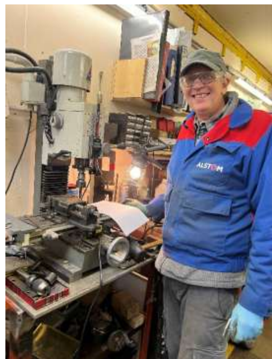
Dave machining a valve for the steam operated drain cocks.
