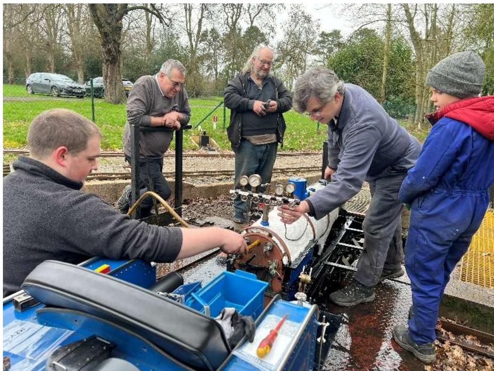
Conor lighting a fire to assist the descaling of the boiler
