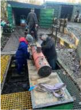
Logan and John starting to descale the boiler.
