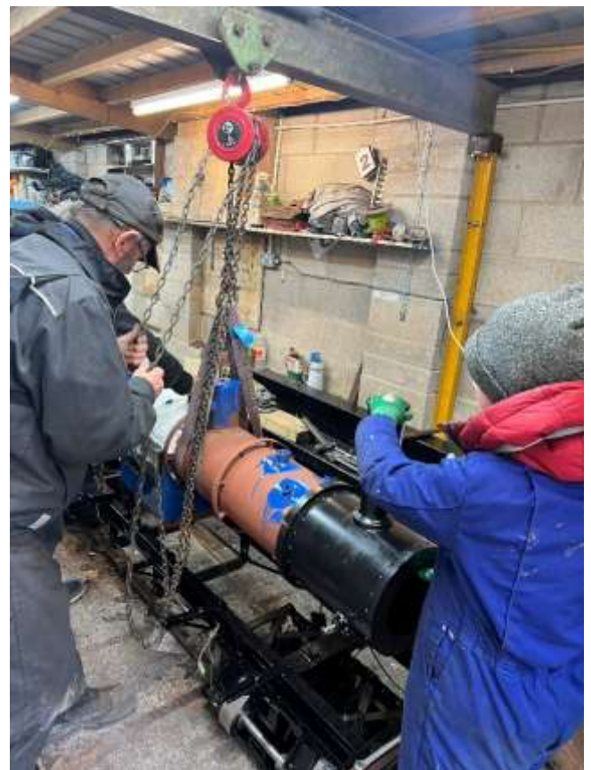
Logan, Phil and John craning and fixing the boiler back into the chassis.
