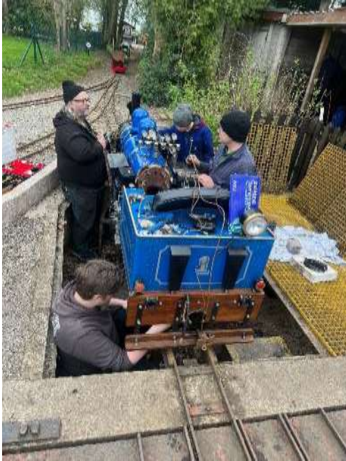
Pipework being reconnected on The Shay
