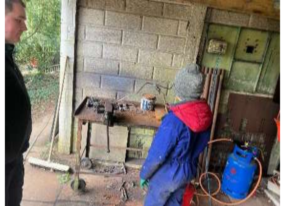
Connor teaching Logan how to anneal pipework so that it can be shaped, and then reconnected to The Shay.
