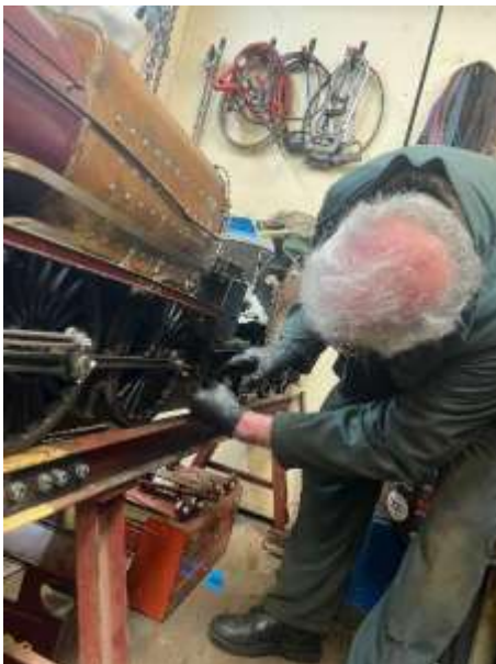
John working on new pipework connectors to the injectors on The Royal Scot. This work will mean that future service work on the injectors will be more accessible and less time consuming.
