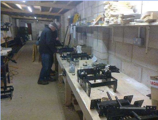
CS2 was used to build new carriages and had a long bench for assembling bogies.
