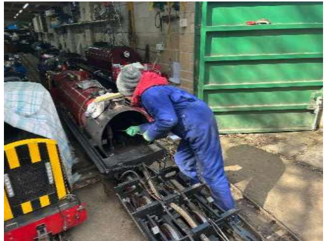
Logan cleaning the boiler tubes in The Garratt, prepping for Public Running.
