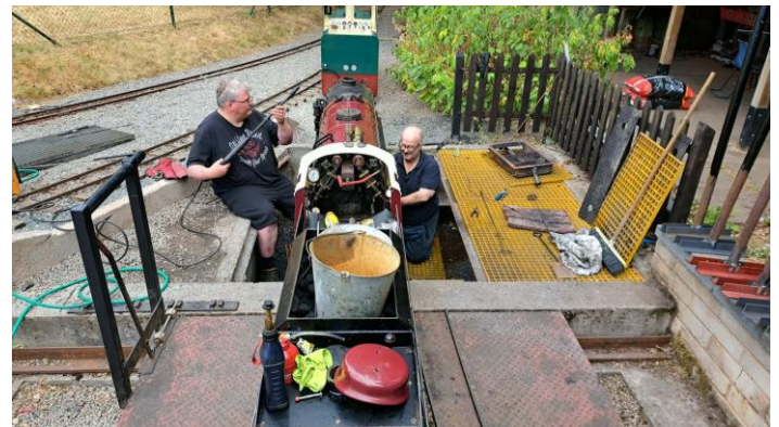
Boiler wash out day for the Garrett.
