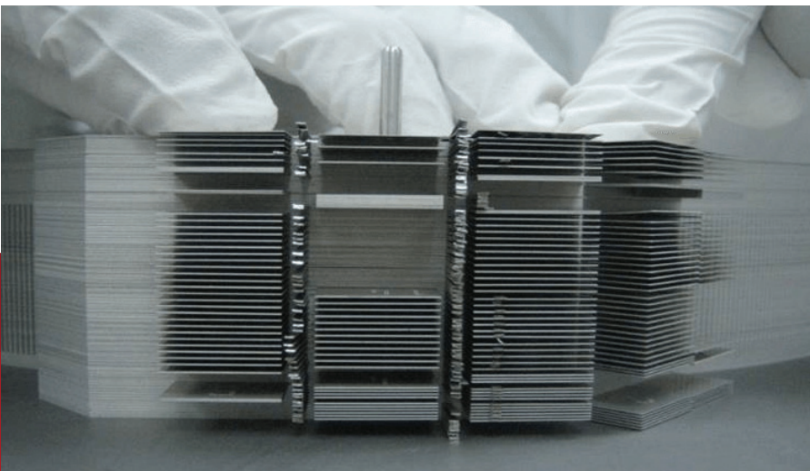
Stacking of CPHX platelets prior to diffusion bonding
