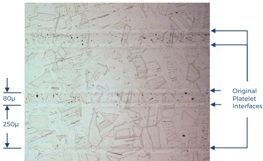
Micrograph of a diffusion bonded 300 series stainless steel part; the microstructure shows grain boundary propagation across the five platelet interfaces
