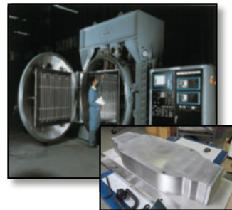
Diffusion Bonding Forms Monolithic Part
