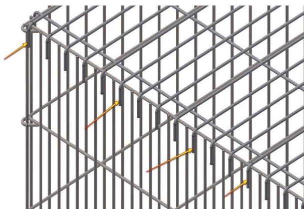
Figure A.15 – Step 13: bend inwards all the 90° laid hooks of the top panel
