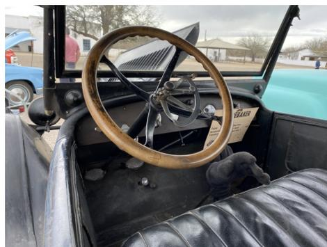
The throttle and timing adjust are on the steering wheel
