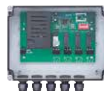
4-channel relay receiver HER 4 BS 4 volt-free relay outputs with status query
