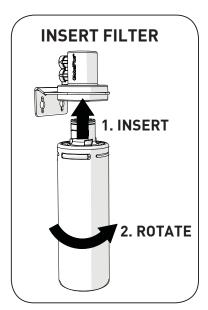
This instruction is for the replacement of the filter in the Zip HydroTap product where the filter is mounted internally. In preparation for your filter flushing, ensure you have a 10 litre container available.
