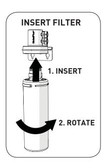
This instruction is for the replacement of the filter in product where the filter is mounted externally. Variations apply depending on the product. Refer to individual instruction. In preparation for your filter activation/flushing, ensure you have a 10 litre container available.
