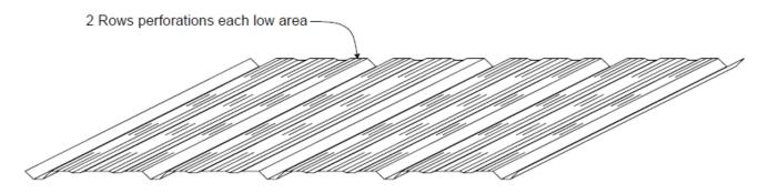
Soffit panel covers 36" and is composed of five inverted ribs, 9" on center and 5/8" deep. The stiffener ribs between the major ribs are symmetrical with the flat areas to provide an attractive appearance. Vented soffit has 9.64 sq. inch of airflow. The paint coating on the NorStar panel is a high quality SMP (Silicone Modified Polyester) finish.
