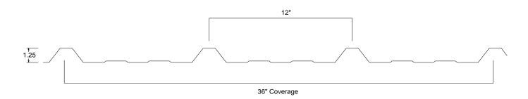
**HUSKY HI-RIB** provides a tough durable wall or roof system and covers 36". It is composed of four major ribs 12" on center and 1 1/4" high. The higher rib provides the extra strength that is needed for longer spans on industrial jobs while creating an attractive, clean appearance.
