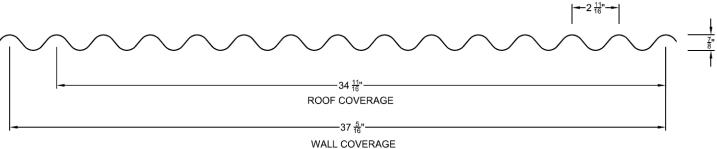
The 7/8" Wave panel provides 37-5/16 inch wall and 34-11/16 inch roof coverage and is composed of major S-shaped ribs at 7/8 inches tall and 2-11/16 inch on center. This product can be utilized as a roofing, liner and/or siding panel. Most commonly it is utilized as a an accent or wainscot panel for interior and exterior walls.
