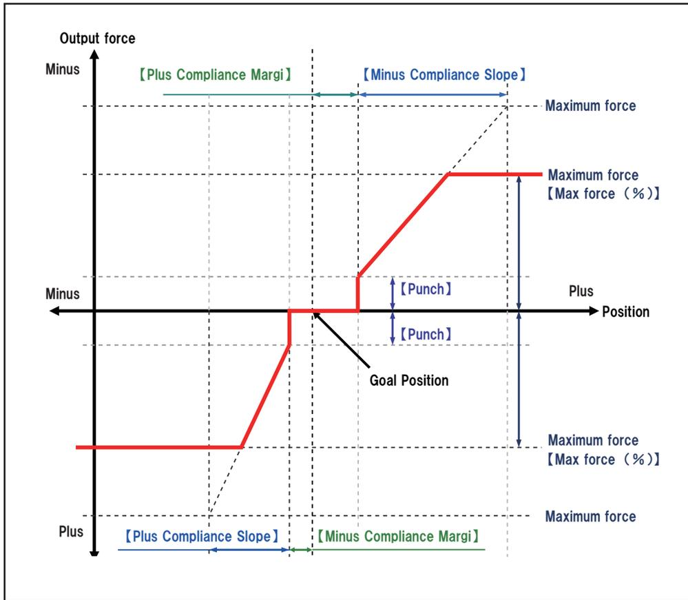
**Fig 4.1 The relationship of Output Force, Position and Compliance settings.**
