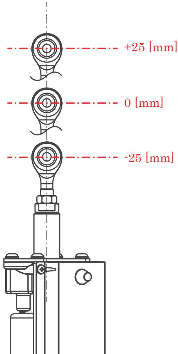
Fig 2.5 Definition of servo stroke positions
