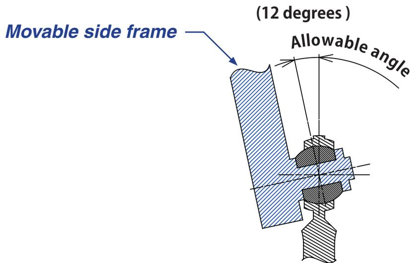
Fig 2.7 Allowable angle of rod end (sectional view)
