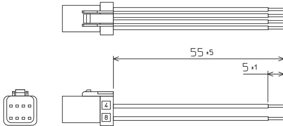
Fig 5.2 LJ9DA41 Cable (unit : mm)
