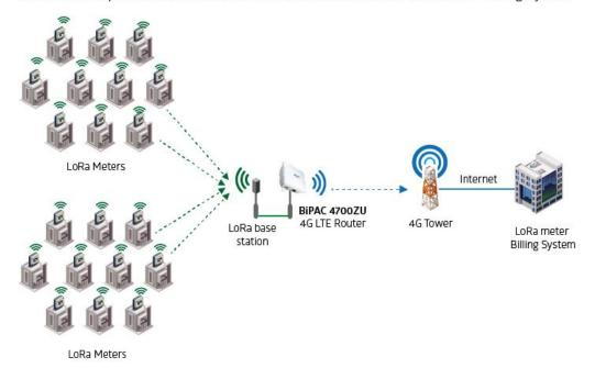
4G LTE Router provides a back haul to connect LoRa meters to LoRa meter Billing System
