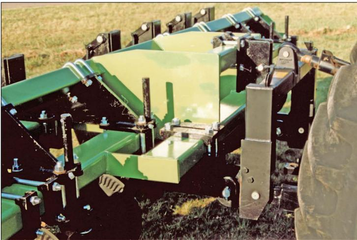
Heavy duty diamond mast frame has 4 x 7 x 3/8" tube on all lower frame members. Optional extended front hitch mount provides flexibility to place coultters and Legs on any row spacing. Heavy Category III Wide 4" Drop Hitch is standard on all models.
