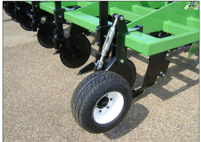
Heavy duty diamond mast frame has 4 x 7 x 3/8" tube on all lower frame members. Optional extended front hitch mount provides flexibility to place coultters and Legs on any row spacing. Heavy Category III Wide 4" Drop Hitch is standard on all models.
