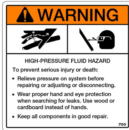
Only adequately trained and qualified persons should work on hydraulics systems. You may be severely injured or killed by being crushed under a falling piece of equipment. Always have transport locks in place and frame sufficiently blocked when working on any implement.
