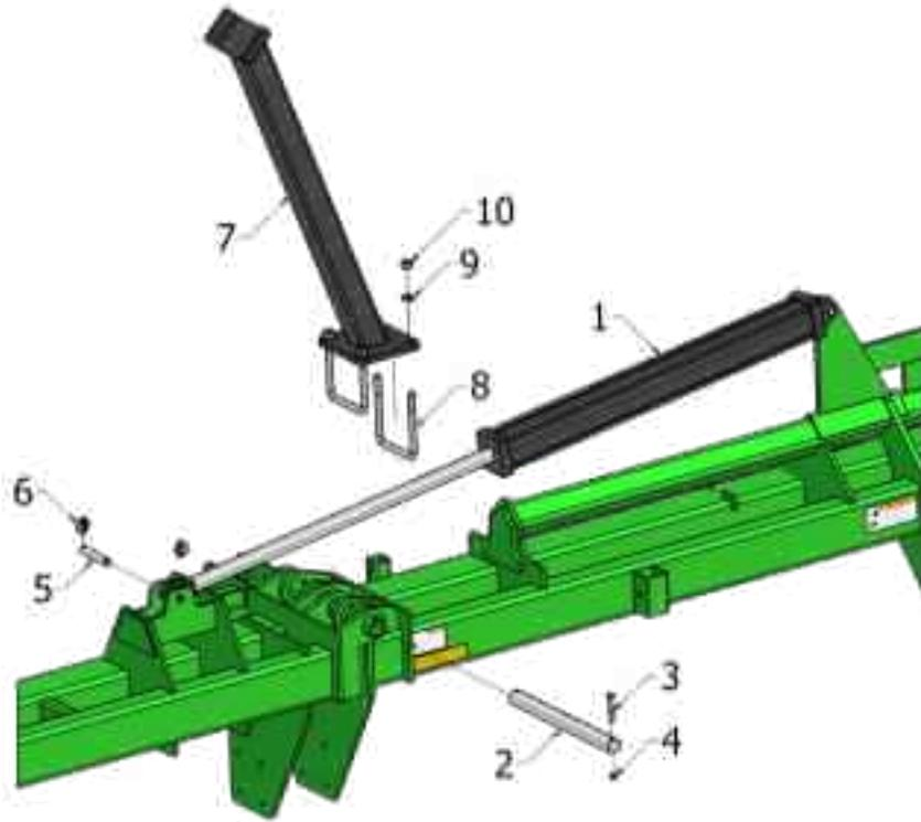
Table 3 – Folding Wing Components for Overfold Units
