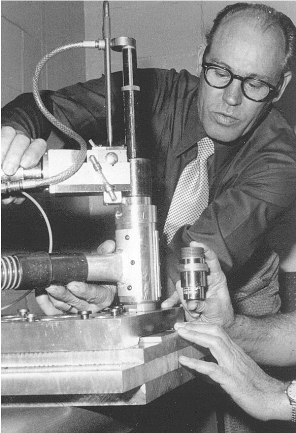
Mr. Ray Culver (Lockheed-Georgia) shown setting up a right angle motor with Portable Gun Drilling Accessories.
