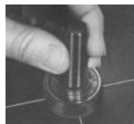
PRECISION CENTER PUNCH INSERTED IN CENTER-RITE BODY
