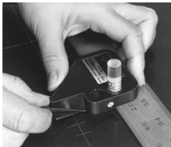
SCRIBE-RITE LAYOUT TOOL WITH OPTICAL CENTERING GAUGE
