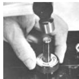
TAPPING HOLE WITH PRECISION CENTER PUNCH THRU
