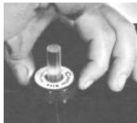
VIEW THRU THE VERTICAL OPTICAL CENTERING GAUGE
