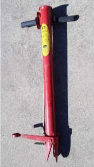
The Pottiputki can reduce bending when planting by sliding tubestock down the barrel of the device. Photo Ruth Aveyard
