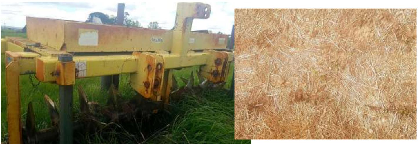
The aerator implement and the deep impressions created when used with the correct amount of soil moisture.
