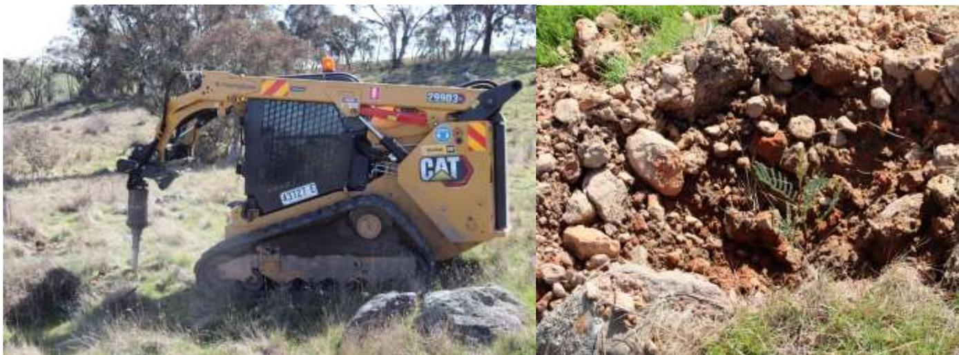
The tracked bobcat in action drilling one of the 10,080 holes and an Acacia seedling freshly planted deep within the hole. Due to the rocky, granite based country some machinery repairs were necessary. Photo: Colin Price and Emily Clarke
