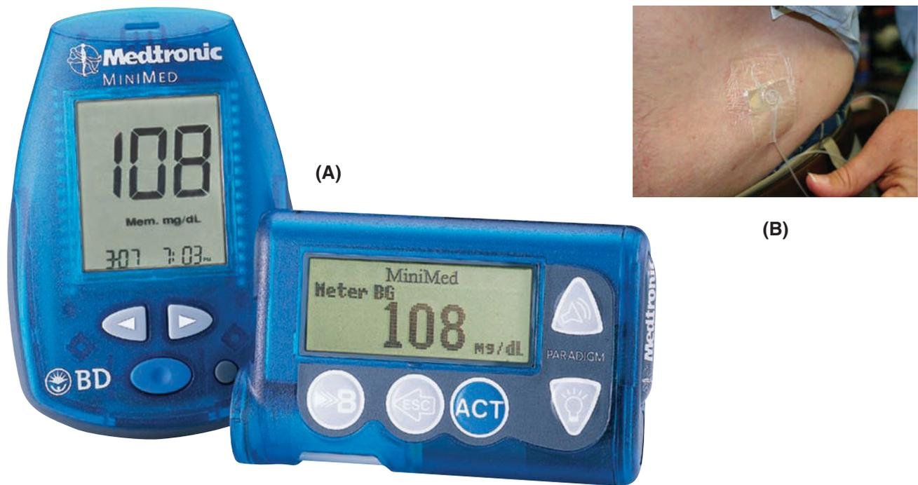
**Figure 13-13A and B** An example of an insulin pump: (A) insulin pump, (B) insulin pump attached to abdomen. (Courtesy of F. Caldwell)
