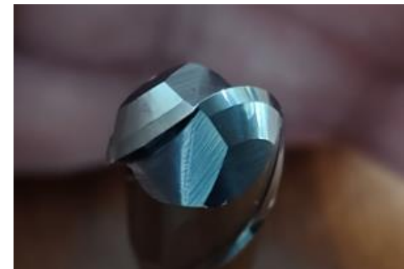
Figure 4: Image of the Tool After 12 Hours of Machining
