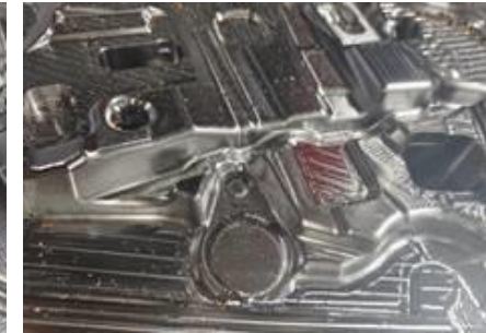
Figure 3: Surface Quality of the Machined Product's Face and Sidewall
