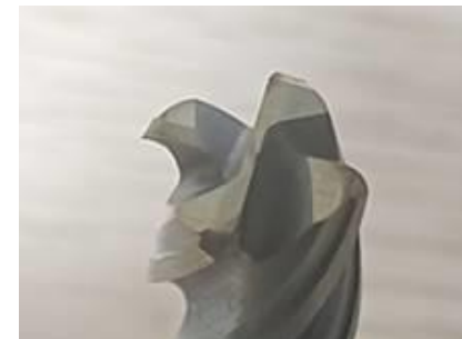
Figure 4: Tool Corner Slight Wear After 19 Hours of Machining
