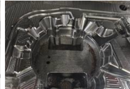
Figure 2: Surface Quality of the Machined Cavity Sidewall
