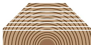
The halved log is sliced straight across. The cut runs parallel to a line through the centre of the log, and at a tangent to the growth rings.
