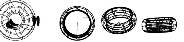
Figure 1 - skewed torriod for the cmc joint created with swept surfaces. The location of the axes determines the surface saddle shape.
