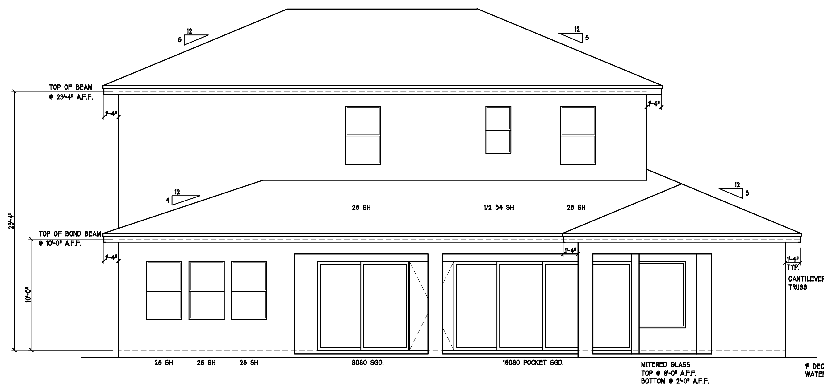
REAR ELEVATION: "F" SCALE: 3/16" = 1'-0"
