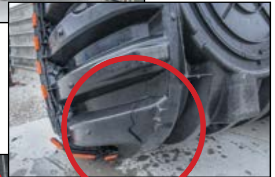
Tank cracked, clips on seam were dislodged.
