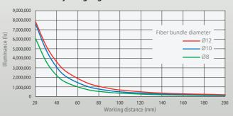
\* Measured at each of the above given distance from fiber end faces of 1080-mm long straight light guides (Ø8 mm, Ø10 mm and Ø12 mm)at 100% illuminance (Not guaranteed)
