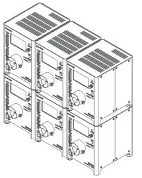
\* Stacking one SLG-150V on top of another is possible only in proper operating environments.
