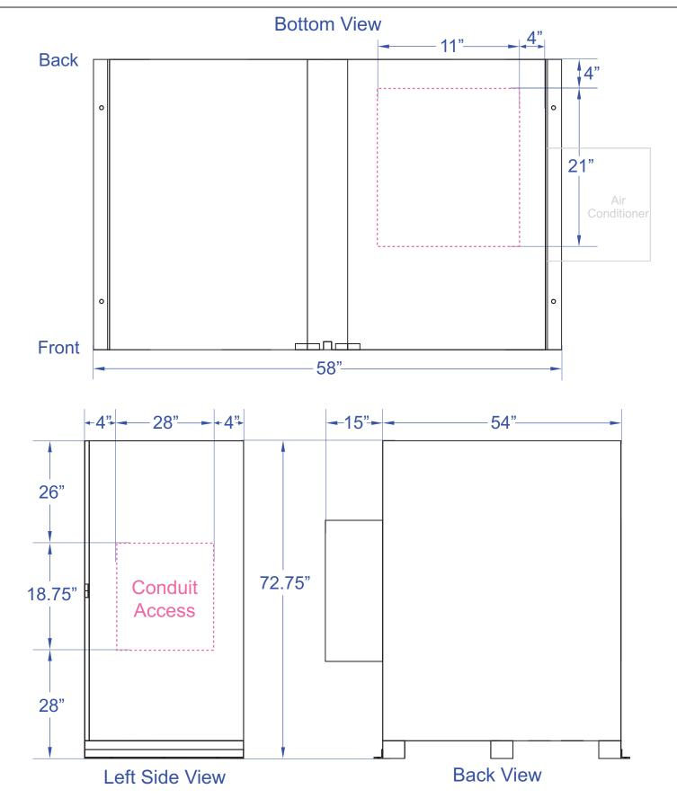
Per code requirements please leave 3" on each side of the cabinet including the back, and a 3 foot clearance in front.
