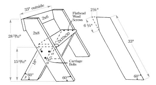
Materials: One 2x6x33", one 2x10x30", one 2x8x10', six ¾"x3½" carriage bolts with washer and nut, twelve ¾"x3½" #12 or #14 flathead wood screws. Use Douglas Fir for your Leopold bench, if you can, and customize its size to suit you. The materials listed will make a 33" bench, but you may choose to build out to 48".
