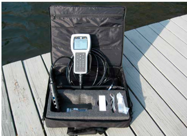
Figure 2 Portable dissolved oxygen meter 1
