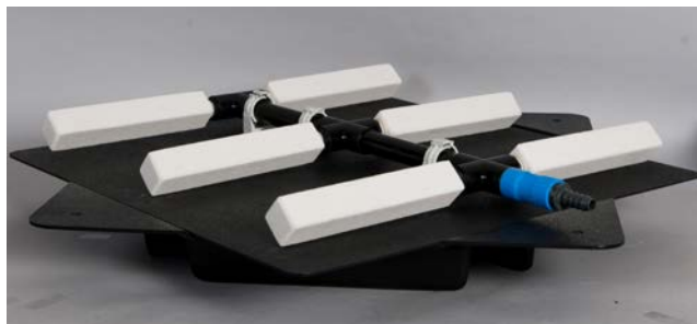
Figure 8 Example diffuser with six individual silica air stone mounted on bottom of plate 1
