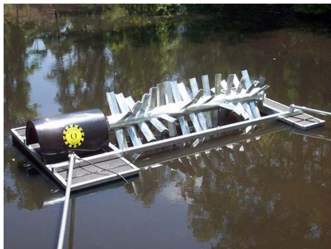
Figure 7 Electric paddle wheel aerator 1
