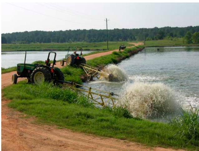
Figure 10 Tractor-driven emergency paddle wheel aerators
