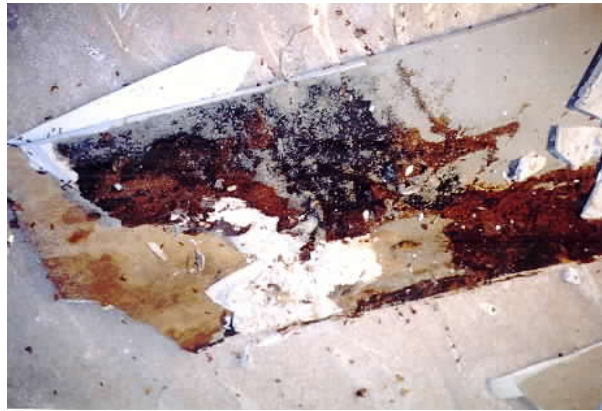
A moldy and ant-infested chunk of wallboard from the writer's house.
