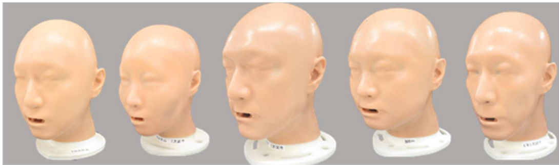
Figure 5. Five soft headforms representing the medium, and four facial categories based on the specified PCA panel, for Japanese workers. (from left to right: Medium, Small, Large, Short-Wide, and Long-Narrow)
