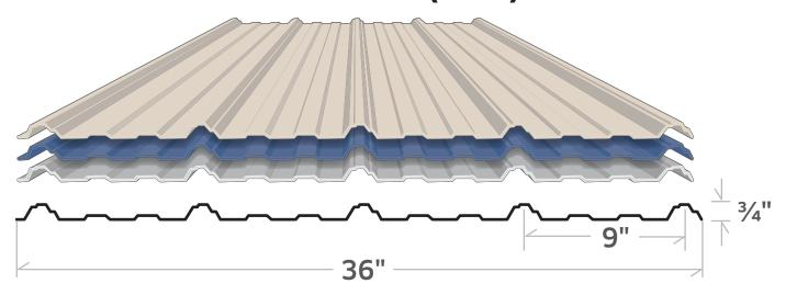
Min Roof Slope: 1/2:12 - 2:12 with Lap Sealant 3:12 and above without sealant
