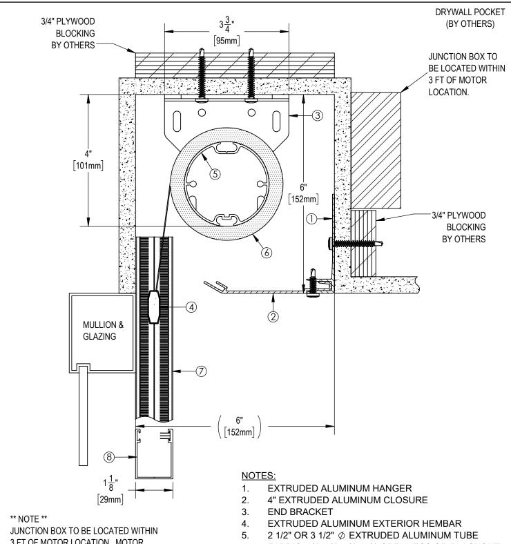
3 FT OF MOTOR LOCATION. MOTOR LOCATION TO BE DETERMINED WITH SOLARFECTIVE REPRESENTATIVE.
