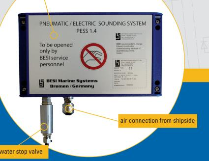
The versatile **PESS** sensor system provides The **PESS** sensor system consists of a readyassembled and pre-adjusted sensor box with an air-throttle valve, a non-return valve, an electronic pressure transmitter, a stop-cock and a test connection for testing the sensor even when the tank is empty.
